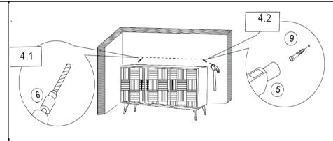
4.1) Drill two holes on wall at same height as Bracket (7) on Sideboard (A) with the Power Drill (6).
