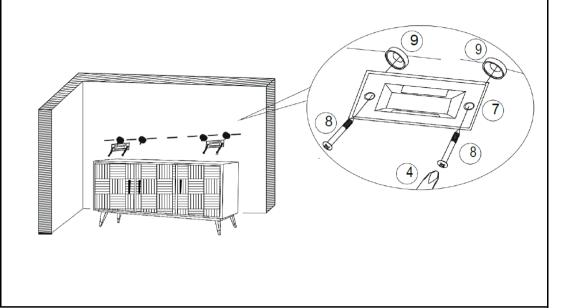
Attach Brackets (7) to Wall Plugs (9) using Wall Plug Screws (8) with Screwdriver (4).
