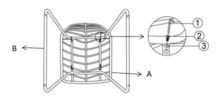
Attach the Legs (B) to Seat (A) using Bolts (②) and Washers (③) with Allen Key (①) as shown in the picture.
