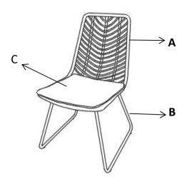
Put the Cushion (C) onto the Chair. Then tie the rope on the Cushion (C) to the seat (B).
