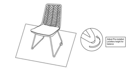
Place the Chair on a LEVEL SURFACE to check for wobbles. If it wobbles, adjust the Legs Pre-installed Levellers until the Chair is level with the ground.
