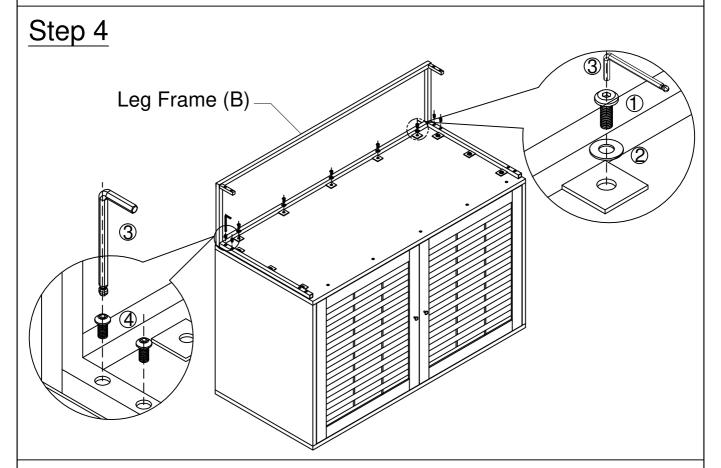
Tighten the Pan Head Allen Bolt (4) & Flat Head Allen Bolt (1) with Washer (2) with the help of Allen key (3).
