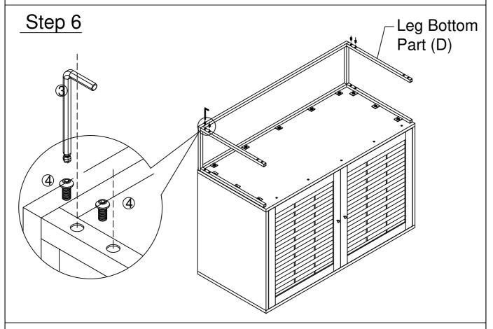
Tighten the Pan Head Allen Bolt (4) with matching holes with the help of Allen key (3).
