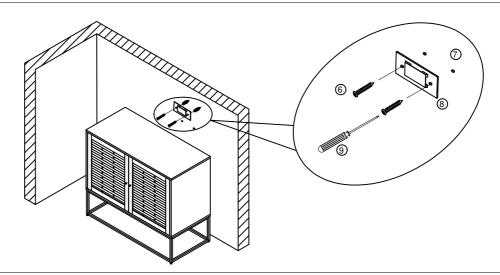
Attach Brackets (8) to Wall Plugs (7) using Wall Plug Screws (6) with Screw driver (9).
