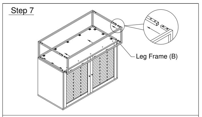
Insert the Leg Frame (B) with matching holes
