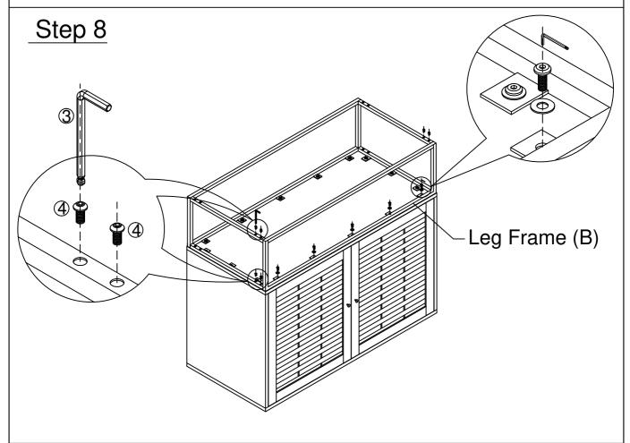
Tighten the Pan Head Allen Bolt (4) & Flat Head Allen Bolt (1) with Washer (2) in matching holes with the help of Allen key (3).
