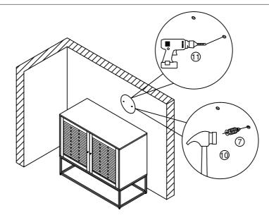
9.1) Drill two holes on wall at same height as Brackets ((8)) on Cabinet with Power Drill ((11)).
