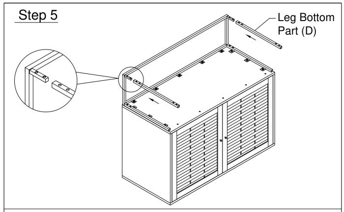
Insert the Leg Bottom Part (D) into Leg Frame (B).
