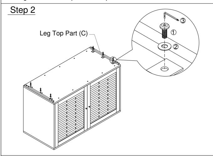
Take the Leg Top Part (C) and tighten it with Flat Head Allen Bolt (1) & Washer (2) with the help of Allen key (3) as shown in the picture above.
