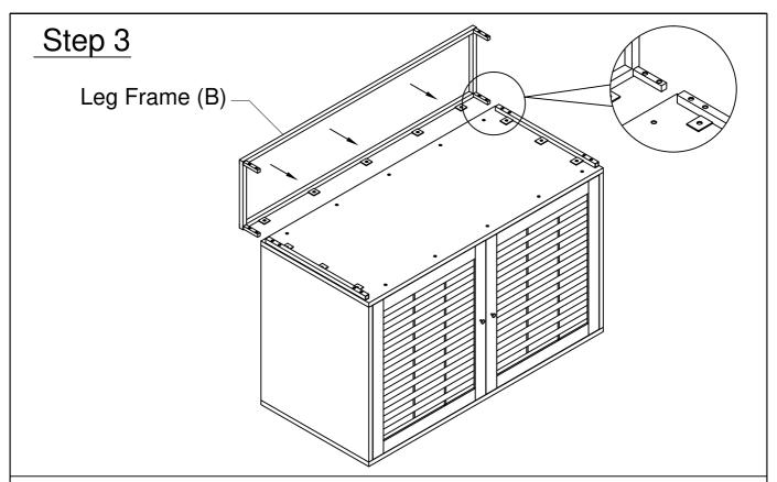
Insert the Leg Frame (B) with matching holes of Leg Top Part (C).
