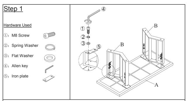
Position the bottom of the Table top(A) as shown.
