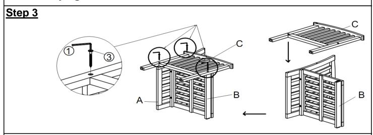
Attach Left Leg Panel (C) to Backrest Panel (A) and Seat Panel (B) using 3 Screws (3) + Allen Wrench (1).
