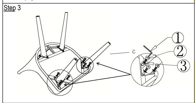
Align the Front Legs(C) with the mounting positions on the base of the Seat(A).
