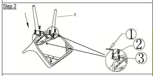
Align the Hind Legs(B) with mounting positions on the base of the Seat(A).
