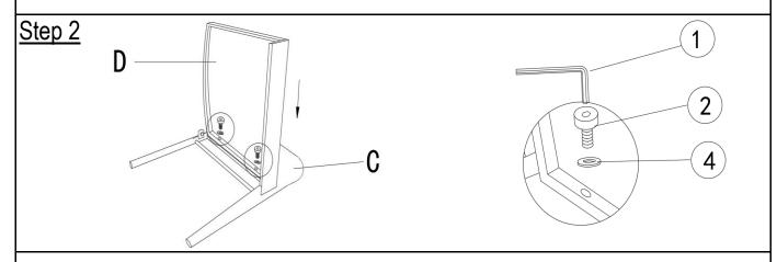
Attach Seat Panel(D) to Right Armrest(C) using Bolts(②) and Washers(④) with Allen Wrench(①). **Do not fully tighten the bolts.**
