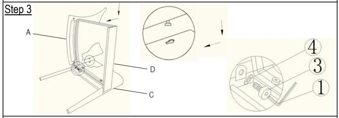
Attach Backrest(A) to Seat Panel(D) and Right Armrest(C) using Bolts(③) and Washers(④) with Allen Wrench(①)
