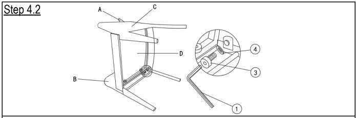
Attach Backrest(A) to Seat Panel(D) and Left Armrest(B) using Bolts(③) and Washers(④) with Allen Wrench(①)
