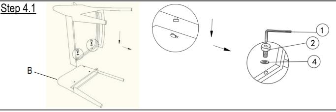
Turn the chair over, and attach the Left Armrest(B) to the Seat Panel(D) using Bolts(②) and Washers(④) with Allen Wrench(①)
