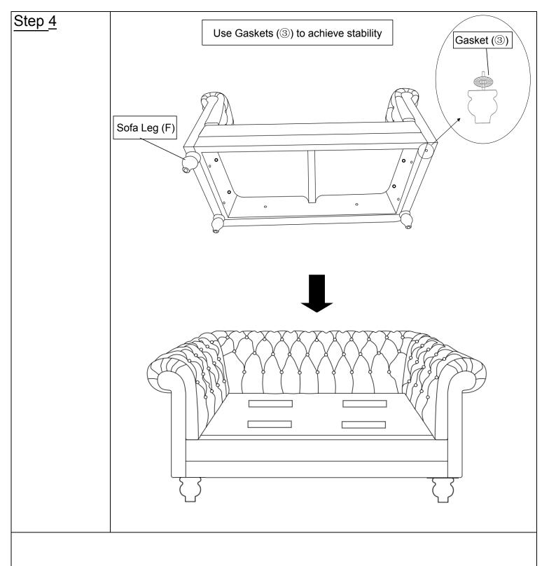
Install the Sofa Leg(F) and the Middle Support Leg(G) onto the bottom of the Sofa by placing one  $Gasket(\ )$  on the threaded stem.
