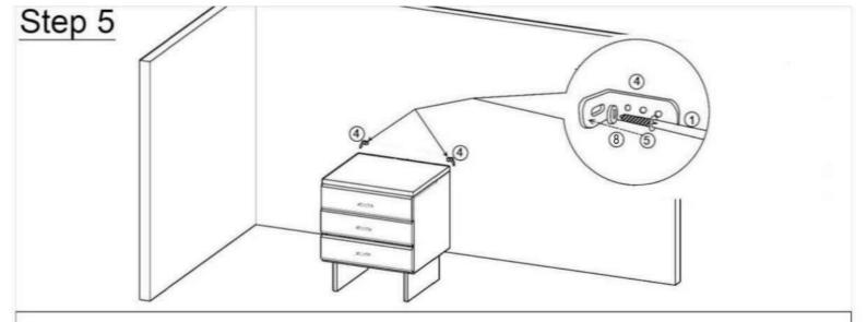
Attach Brackets(4) to Wall Plugs(6) using Wall Plug Screws(5) and Washer(8) with the help of a Screwdriver (1).
