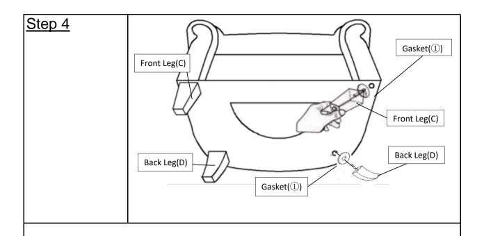
Install Front Leg(C) into the Chair Base(B) by putting a Gasket(①) on the threaded stem. Then insert the threaded stem into the mounting position at the corner of the bottom of Chair Base(B).
