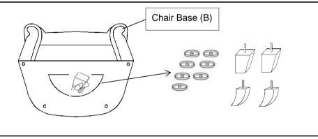
Place the Chair on its back on a clean, non-marring surface as pictured above. Carefully unzip the pouch at the bottom of the Chair Base(B) and remove the Front Leg(C), Back Leg(D) and Hardware.
