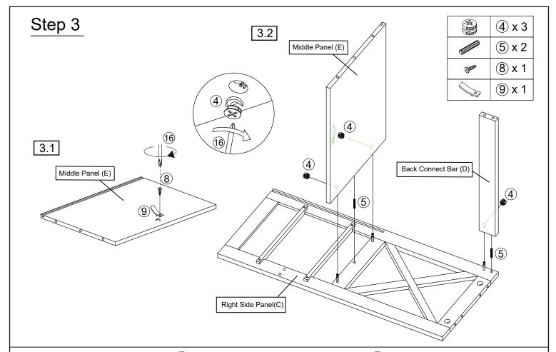
3.1) Attach Drawer Stopper (9) to Middle Panel (E) with Screw (8) using Screwdriver (6).
