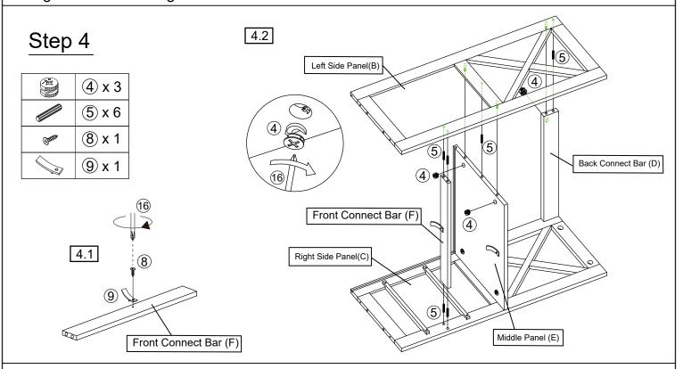
4.1)Attach Drawer Stopper (9) to Front Connect Bar (F) with Screw (8) using Screwdriver (6). 4.2)Attach Front Connect Bar (F) to Right Side Panel (C) with Dowel (5),then attach Left Side Panel (B) to Front Connect Bar (F), Middle Panel (E) and Back Connect Bar (D) with Dowel (5), then insert Cam Nut (4) into Middle Panel (E) and Back Connect Bar (D) using Screwdriver (6) turing clockwise until tight.
