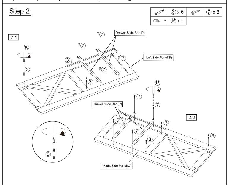
2.1) Attach Drawer Slide Bar (P) to Left Side Panel (B) with Screw (⑦) using Screwdriver (⑥). Insert Cam Bolt (③) into the mounting positions on Left Side Panel (B) using Screwdriver (⑥). 2.2) Repeat the same step with Right Side Panel (C).
