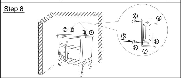
Attach Brackets (7) to Wall Plugs (9) using Wall Plug Screws (8) with Screwdriver (5).
