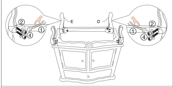
Align the Back Left Leg (D) to the Left side of Cabinet and Back Right Leg (E) to the Right side of Cabinet and attach using the Washer (2) with the Nut (4) and with the help of Spanner (1) as shown in the picture above. Do not completely tighten the Nut.
