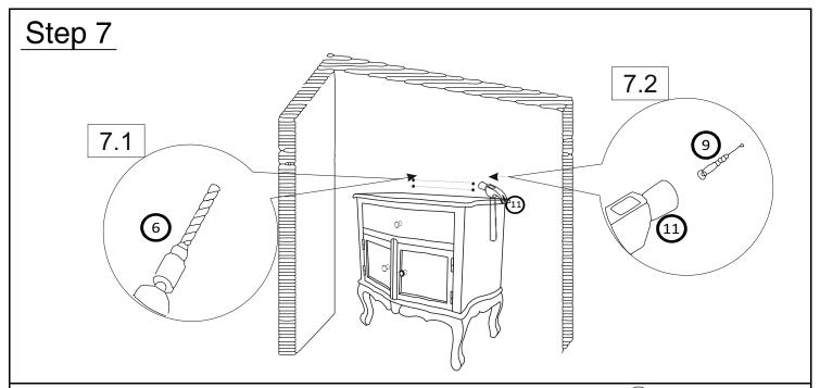
7.1) Drill two holes on wall at same height as Brackets (7) on Cabinet with Power Drill (6).
