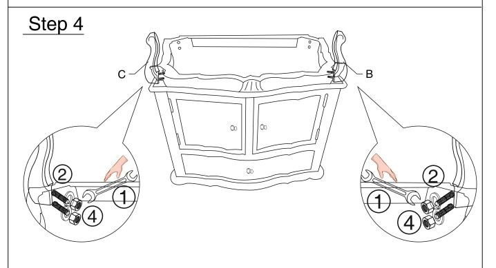
Align the Front Left Leg (B) to the Left side of Cabinet and Front Right Leg (C) to the Right side of Cabinet and attach using the Washer (②) with the Nut (④) and with the help of Spanner (①) as shown in the picture above. Do not completely tighten the Nut.
