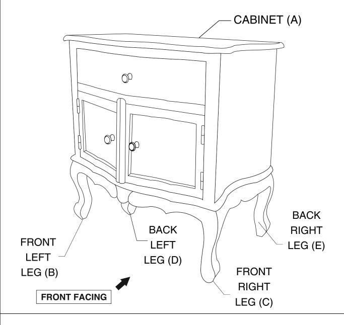
This Cabinet has multiple parts and may require up to some 30 minutes to assemble. To give you an overview of the Cabinet parts, the above picture is to help you put the various parts into perspective. Please read through the instructions below to familiarise yourself with the parts and steps before assembly.
