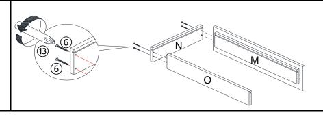
Attach the Drawer Side Panel (N) to the Drawer Front Panel (M) and the Drawer Back Panel (O) using Screws(6) and the Screwdriver(3). **Tighten the Screws fully in a sequential manner.**
