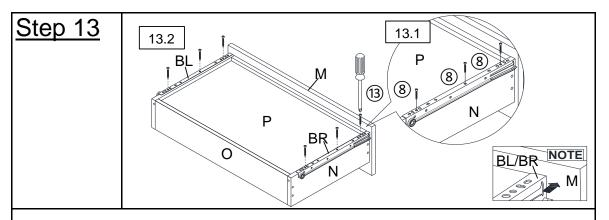
13.1) Attach the Drawer Right Bottom Rail (BR) to the Drawer Side Panel (N) using Screws(8) and the Screwdriver(13) where indicated.
