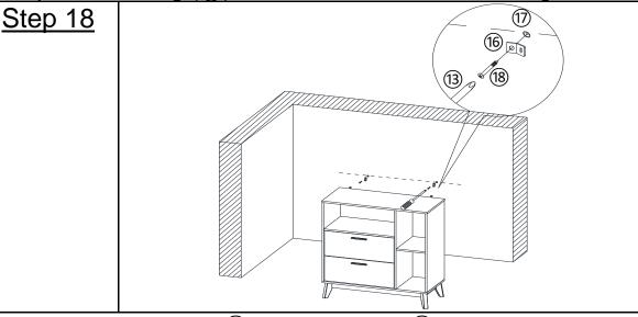
Attach the Metal Brackets(16) to the Wall Plugs(17) using Wall Plug Screws(18) and the Screwdriver(13).
