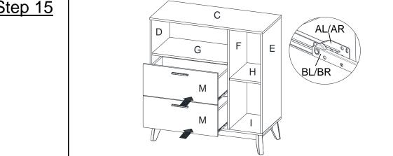
Put the Drawer Assembly in place by aligning the rails.
