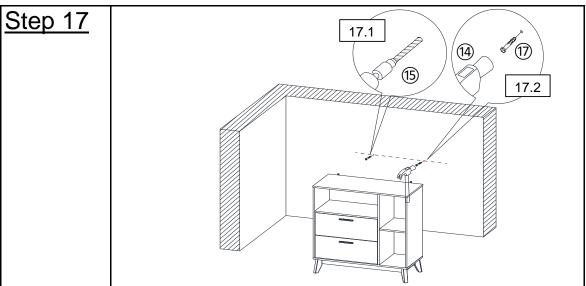
**17.1)** Drill two holes on the wall at the same height as the Metal Brackets(16) on the Cabinet using a Power Drill(15).
