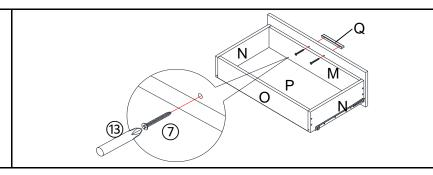
Attach the Handle (Q) to the Drawer Front Panel (M) using Screws(7))and the Screwdriver(13).
