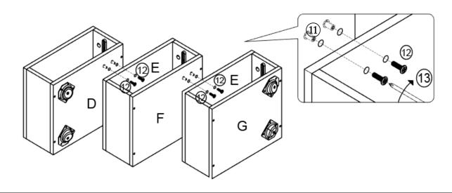
Attach Bolt(①) and Nut(①) to the Upper Bottom Panel(D), Lower Top Panel(E) and Middle Bottom Panel(F) using Screwdriver(③).
