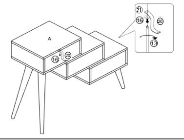
Attach Restraint Strap(②) to the Top Panel(A) using Screw(⑥) and Metal Gasket(②) with Screwdriver(③).
