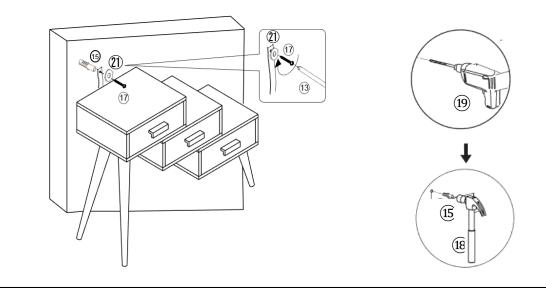
Drill one mounting position on the wall with Power Drill(1), insert Wall Anchor(1) into drilled mounting position on the wall with Hammer(1). Move the cabinet back to the wall, lock by Screw(1) and Metal Gasket(2) with Screwdriver(3).
