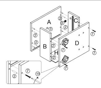
Insert Dowel(②) into the mounting positions on Left Side Panel(B) and Right Side Panel(C), attach Left Side Panel(B) and Right Side Panel(C) to the Top Panel(A), insert Cam Nut(③) into the mounting positions on Left Side Panel(B) and Right Side Panel(C) locked by Screwdriver(③).
