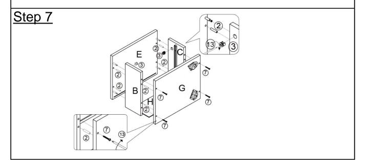
Insert Dowel(②) to the mounting positions on Left Side Panel(B) and Right Side Panel(C). Attach Left Side Panel(B) and Right Side Panel(C) to the Lower Top Panel(E), insert Cam Nut(③) into the mounting positions on Left Side Panel(B) and Right Side Panel(C) locked by Screwdriver(③).
