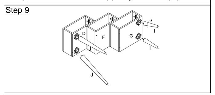
Attach two Left Leg(J) to the Upper Bottom Panel(D), then shift them tightly by hands. Attach two Right Leg(I) to the Lower Bottom Panel(G), then shift them tightly by hands.
