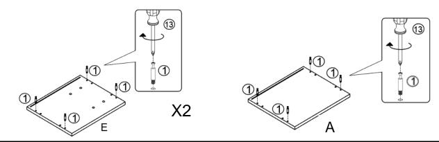
Insert Cam Bolt(1) into the mounting positions on Lower Top Panel(E) and Upper Top Panel(A) using Screwdriver(13).
