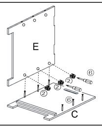
Attach Back Panel(E) to the Cam Bolt on Left Side Panel(C) using Cam Nut(2) with Screwdriver(6) as shown.
