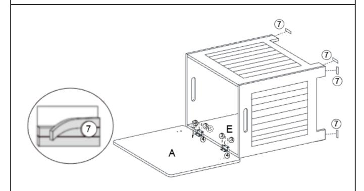
Attach Hinge(4) to the Back Panel(E) and Top Panel(A) using Screw(3) with Screwdriver(6) as shown.
