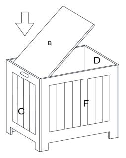
Insert Bottom Panel(B) into the Cabinet at a 45° angle.
