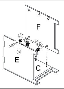
Attach Front Panel(F) to the Cam Bolt on Left Side Panel(C) using Cam Nut(2) with Screwdriver(6) as shown.
