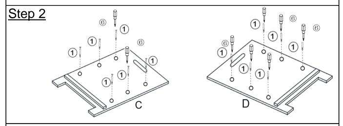
Attach Cam Bolts(1) to the Left Side Panel(C) and Right Side Panel(D) using Screwdriver(6) as shown.
