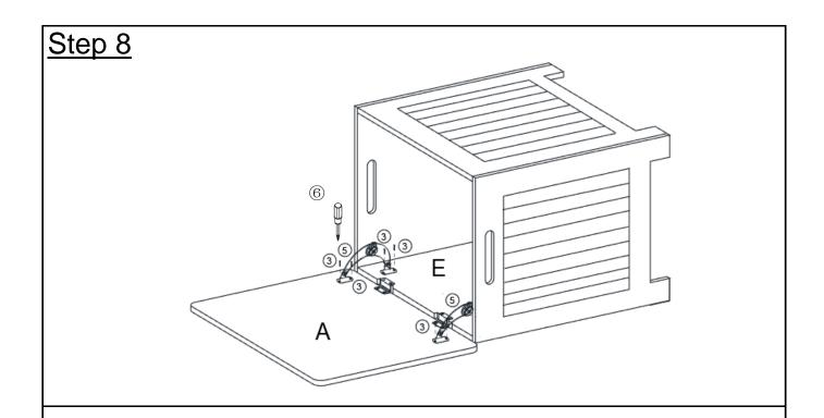
Attach Lifting Arm(⑤) to the Top Panel(A) and Back Panel(E) using Screw(③) with Screwdriver(⑥) as shown.
