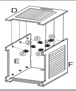
Attach Right Side Panel(D) to the mounting positions on Front Panel(F) and Back Panel(E) using Cam Nut(2) with Screwdriver(6).
