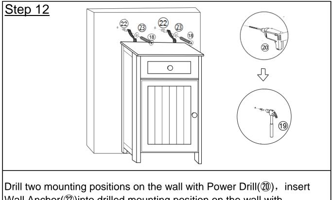
Wall Anchor((22)) into drilled mounting position on the wall with Hammer((19)). Move the cabinet back to the wall, lock by Screw((18)) and Metal Gasket((23)) with Screwdriver((14)).
