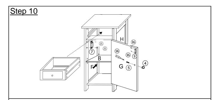
Attach Door Knob((4)) to the Door Panel(G) using Screw((5)) with Screwdriver((4)).
