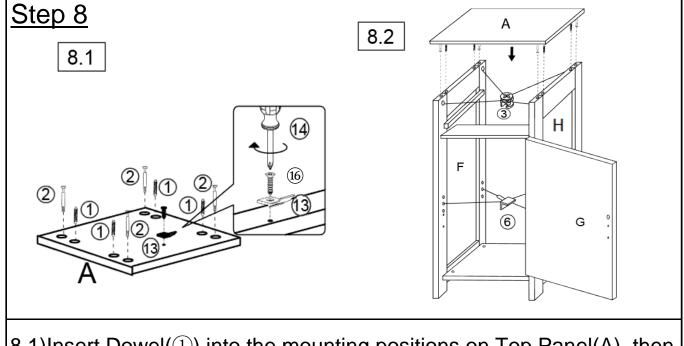
8.1)Insert Dowel(1) into the mounting positions on Top Panel(A), then attach Cam Bolt(2) to the mounting positions on Top Panel(A) using Screwdriver(1) as shown. Attach Stoper(1) to the Top Panel(A) using Screw(1) with Screwdriver(1).
