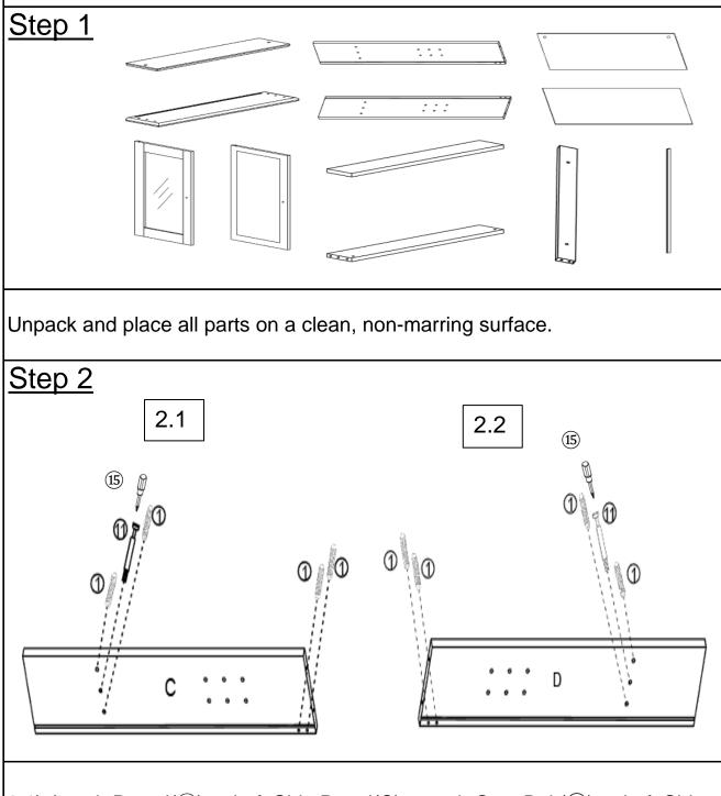
2.1) Attach Dowel(1) to Left Side Panel(C), attach Cam Bolt(11) to Left Side Panel(C) Using Screwdriver(15) as shown.
