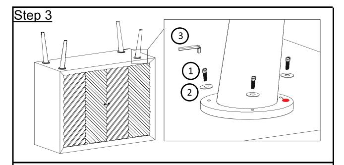
Place the Cabinet (A) upside down onto a clean, soft surface to avoid any scratches or damages to the product. Align the holes of Cabinet (A) into all Legs (B) as shown above. Match the red sticker.
