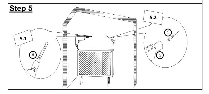
5.1) Drill two holes on wall at same height as Brackets (①) on cabinet with Power Drill (⑥).
