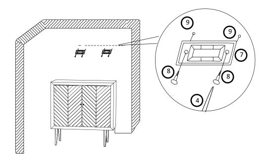
Attach Brackets (7) to Wall Plugs (9) using Wall Plug Screws (8) with Screwdriver (4).
