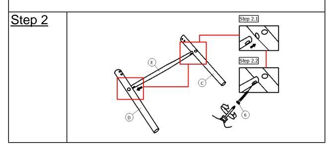
**2.1)** Insert the Front Rail(E) into the oval housings of Front Leg(C) and Front Leg(D) as shown above.
