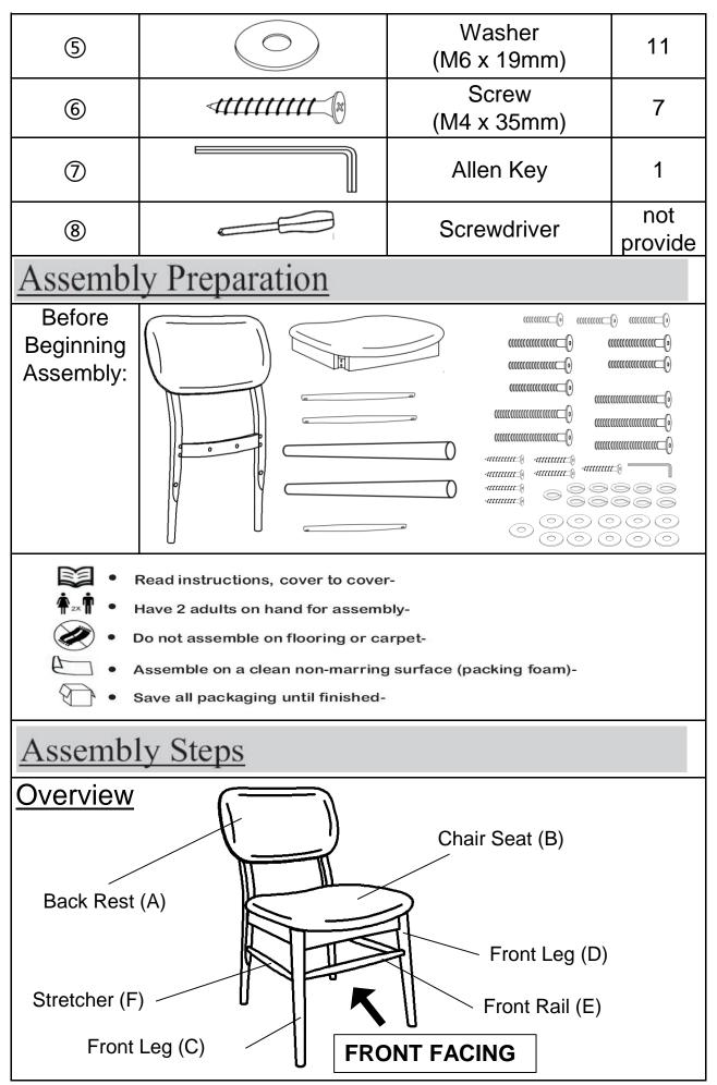
This Chair has multiple parts and may require up to 30 minutes to assemble. To give you an overview of the Chair parts, the above picture is to help you put the various parts into perspective. Please read through the instructions below to familiarise yourself with the parts and steps before assembly.
