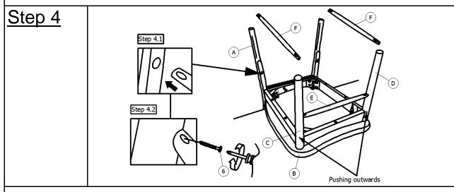
4.1) Place Stretchers(F) into housings between the hind legs of the Back Rest(A) and Front Leg(C) and Front Leg(D).
