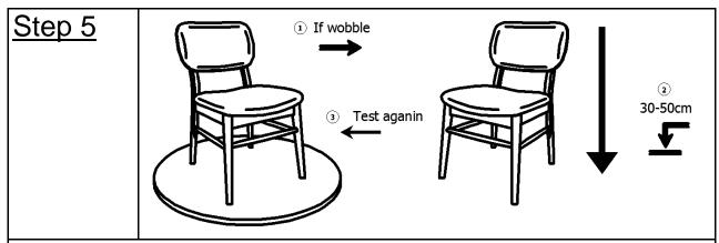
Place the Chair on a Level Surface to check for wobbles. If there are wobbles, lift the Chair some 30cm to 50cm high from the ground, keep your feet and toes away form the drop zone, and drop the Chair vertically with all four legs, hitting the ground at the same time. The Drop Test will help to ensure that all Screws, Bolts and gaps reach full alignment. Test again for evenness on a Level Surface.
