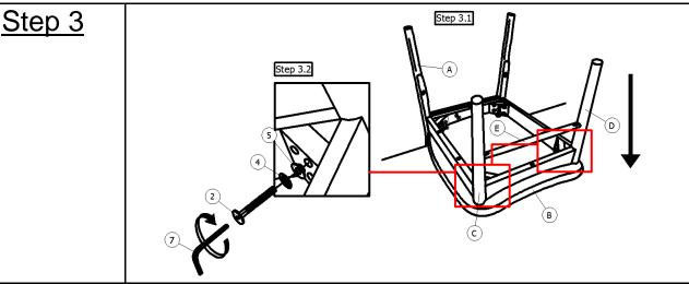
**3.1)** Place the Chair on the edge of a table, as shown. Then insert the Front Legs(C&D) into the bottom of the Chair Seat(B).
