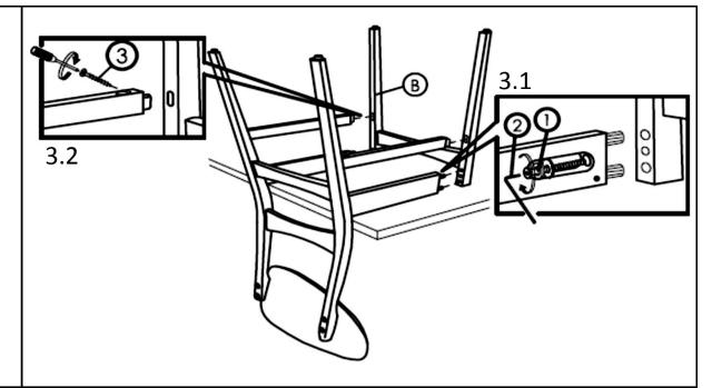
Insert Front Leg(B) onto the Side Stretchers and Side Rails as shown.
