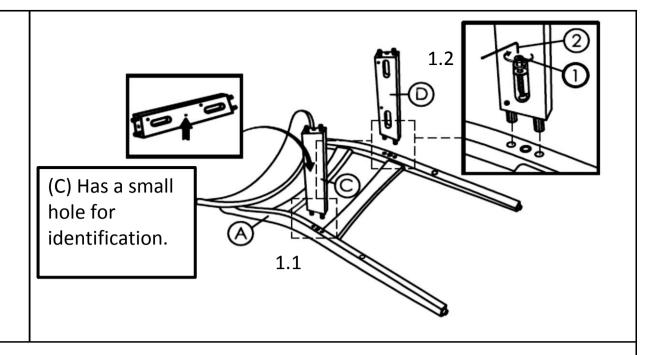
**1.1)** Insert the Side Stretcher(C) and Side Stretcher(D) into the Chair Back(A) as shown.
