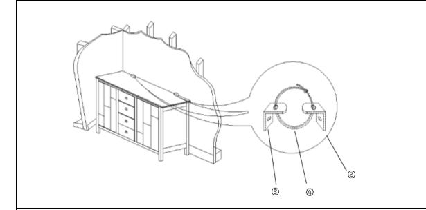
**C:** Move the Cabinet against the wall. Then pull the Cabinet Restraint Strap(4) through two Metal Brackets(3) one by one, lock tight the Cabinet Restraint Strap(4), as shown above. Cabinet Restraint Device is installed and Cabinet is ready for use. Caution: This Cabinet can only be used on a flat, level surface.
