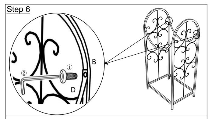
Repeat Step 5 to assemble Left Frame(A) and Right Frame(B) using Bolt(1) with Allen Key(2). Tighten all bolts.
