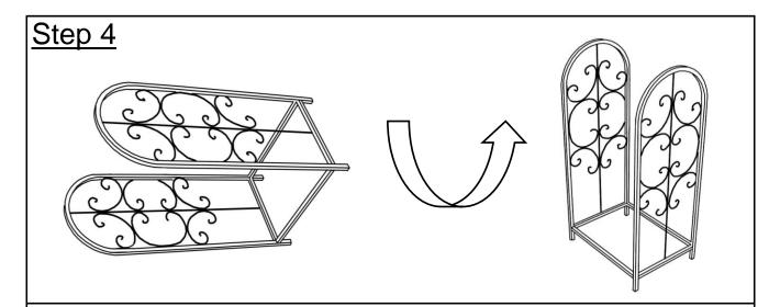
Place the pre-attached frame face up as shown.
