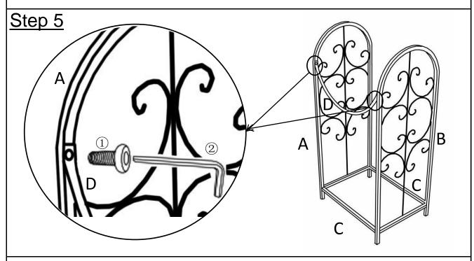
Attached Connect Bar(D) to Left Frame(A) and Right Frame(B) using Bolt(1) with Allen Key(2). Loosely tighten bolts .
