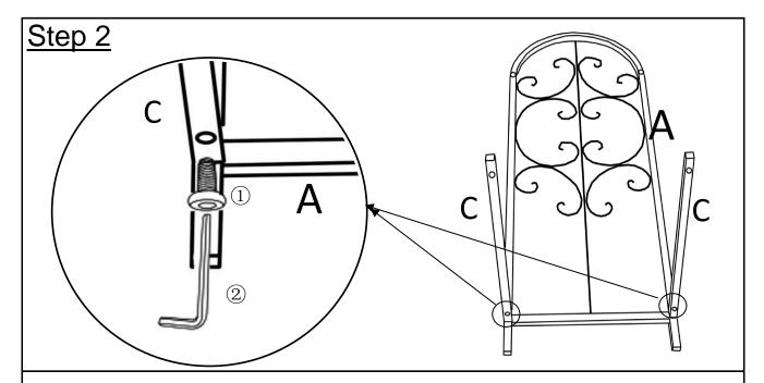
Attached Support Bar(C) to Left Frame (A) using Bolt(1) with Allen Key(2).
