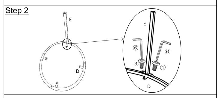
Place Table Top(D) facedown on non-marring surface. Loosely attach Leg(E) to Table Top(D), using Bolt(4) with Allen Key(6) Loosely tighten the Bolts.
