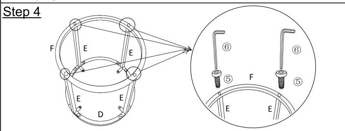
Place the Base(F) into the Legs(E), using Bolt(⑤) with Allen Key(⑥) as shown in picture.
