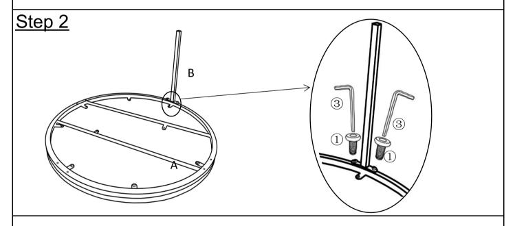
Place Table Top(A) facedown on non-marring surface. Loosely attach Leg(B) to Table Top(A), using Bolt(1) with Allen Key(3) **Loosely tighten the Bolts.**
