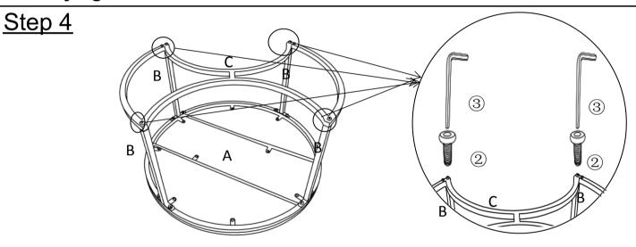
Place the Base(C) into the Legs(B), using Bolt(②) with Allen Key(③) as shown in picture.
