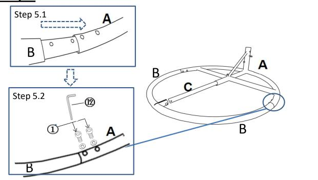
Repeat Step 4, attach another piece of Base Booms - Curved (B). **Don't Fully tighten the bolts in this step.**
