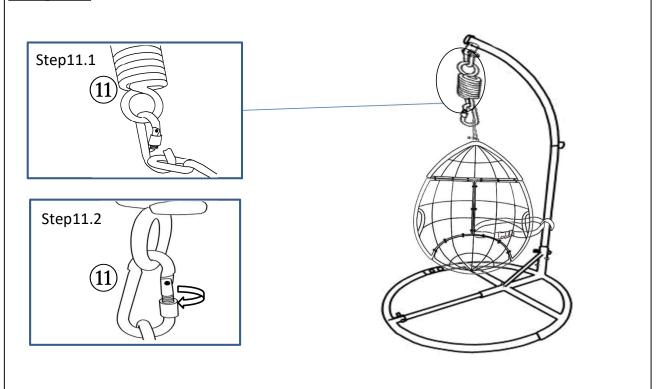
Lift the Basket and hang the Iron Chain on the Spring of the Hanging Chair Base. And Screw the Safety lock tightly.
