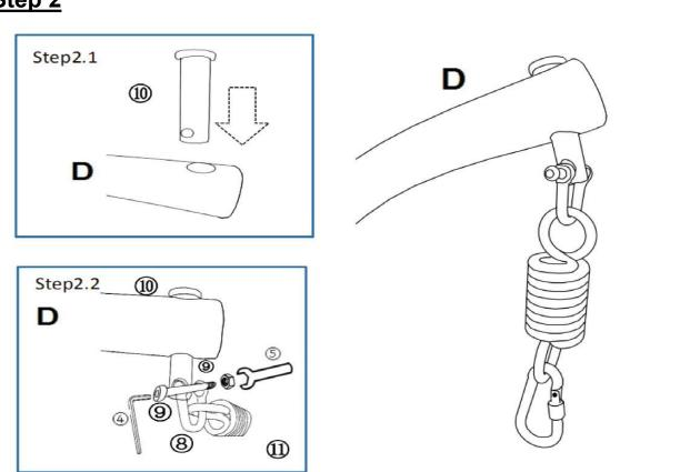
Step 2.1: Attached Bolt(®) to Bent Metal Holder(D).
