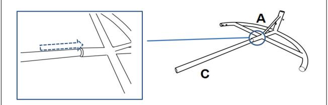
Attached Base Straight Boom Loosely (C) to Base Loosely (A).
