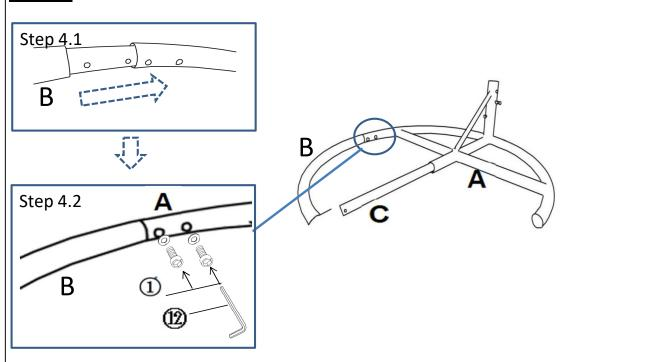
Attached Base Booms - Curved (B) to Base Loosely (A) using bolts and washer (①) with Allen Wrench (②).
