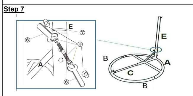
Attached Straight Metal Holder (E) to Base Loosely (A) using Wrench (⑤) with Nuts set (③). Then, Move the Rubber Ring(⑦) down the Lower Pole(E) until it is flush with the top of the Base(A).
