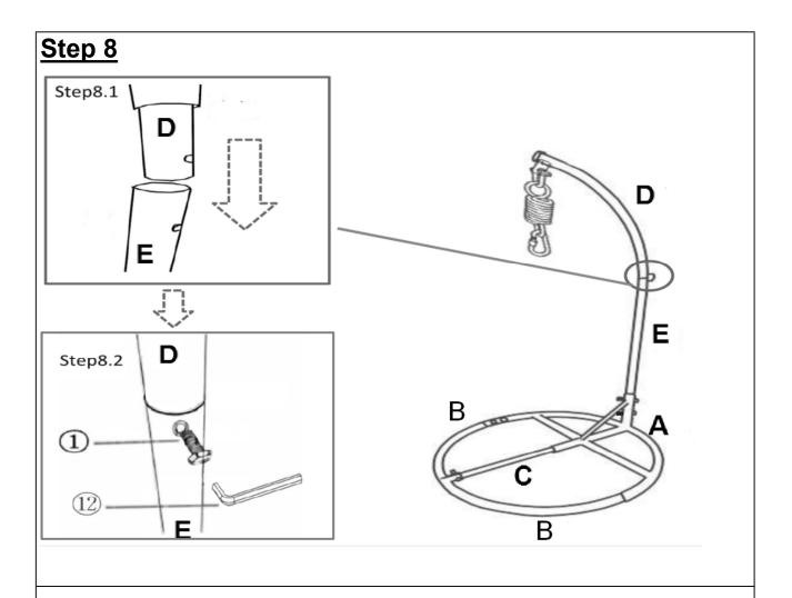
Attached Bent Metal Holder (D) to Straight Metal Holder (E) using Wrench (⑤) with bolt and washer(⑥).
