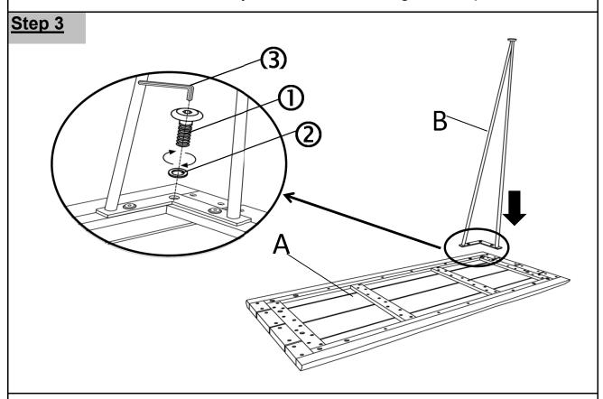
Insert one of legs (B) into the table top (A), put the flat washer (2) and bolt (1) as above picture.
