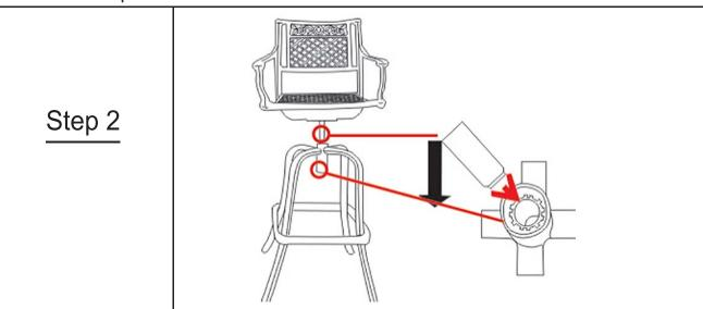
Attach the Seat with attached Iron Plate to the Chair Leg Base as pictured above.
