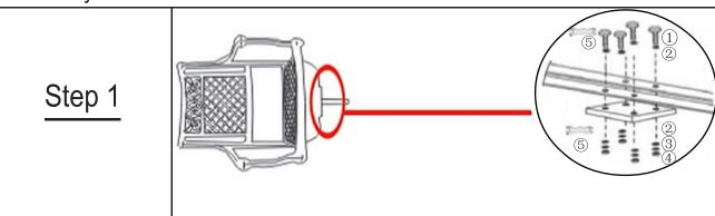
Attach the Iron Plate to the Seat.
