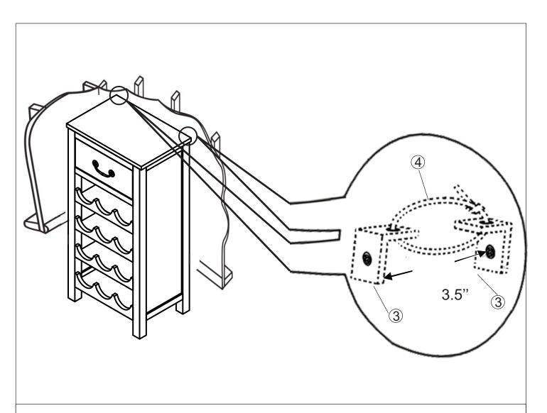
**C**: Move the Cabinet against the wall. Then pull the Cabinet Restraint Strap (4) through two Metal Brackets (3) one by one, lock tight the Cabinet Restraint Strap (4) as shown above.
