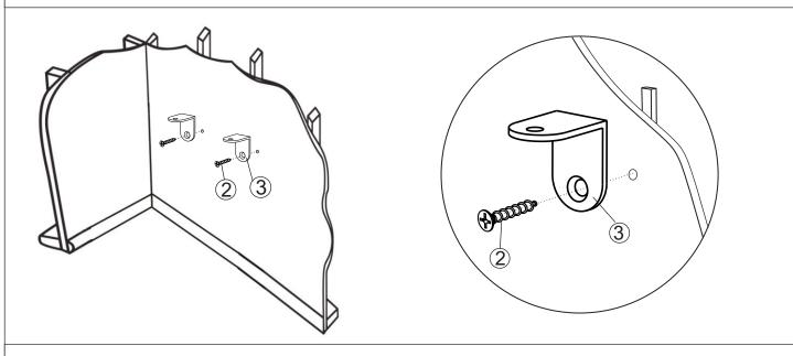
**B:** Find out the screw holes on the wall.
