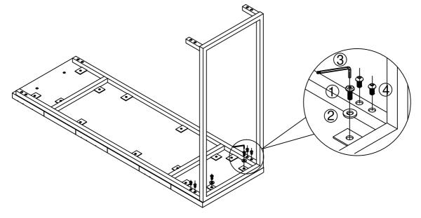
Tighten the Pan Head Allen Bolt (4) with using Allen Key (3). Tighten Flat Head Allen Bolt (1) with Washer (2) with the help of Allen key (3).
