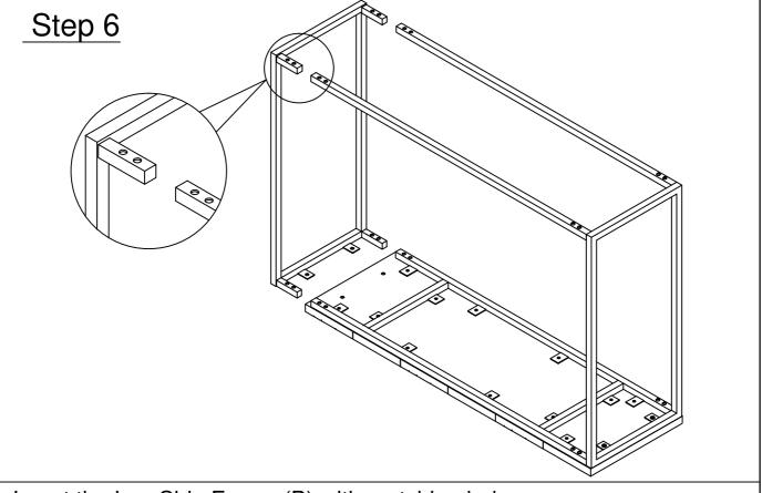
Insert the Leg Side Frame (B) with matching holes
