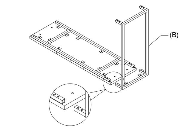
Insert the Leg Side Frame (B) with matching holes of Top Frame (A).
