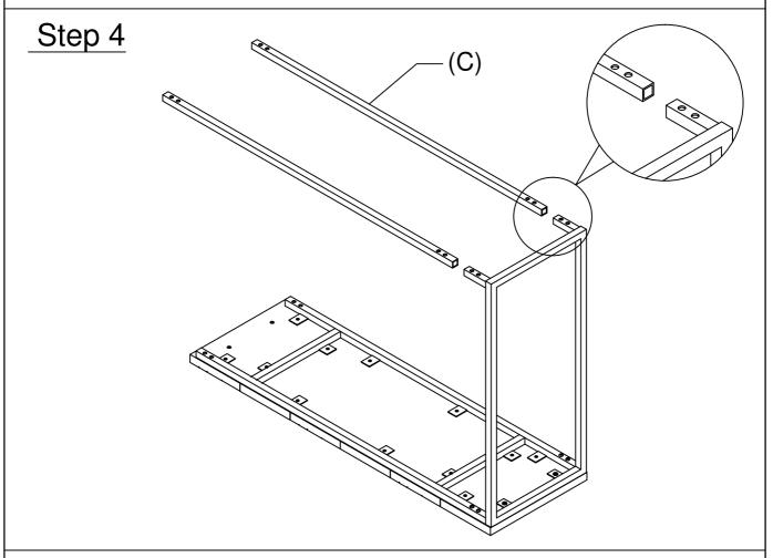
Insert the Leg Bottom Part (C) into Leg Side frame (B).
