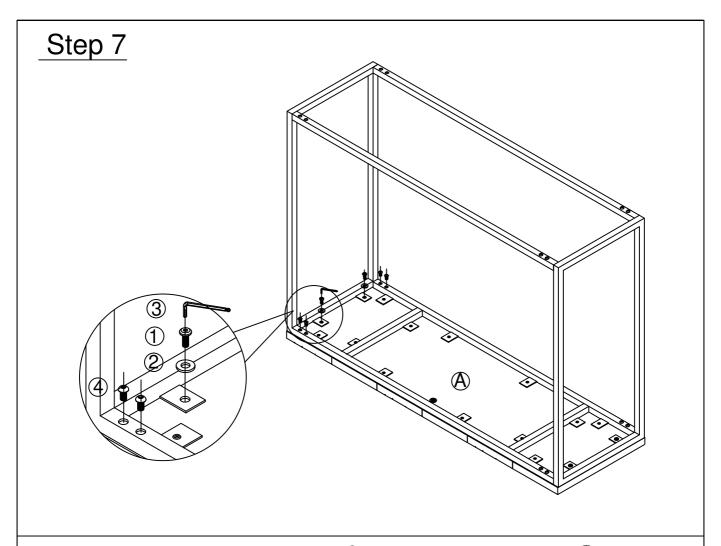
Tighten the Pan Head Allen Bolt (4) with using Allen Key (3). Tighten Flat Head Allen Bolt (1) with Washer (2) with the help of Allen key (3).
