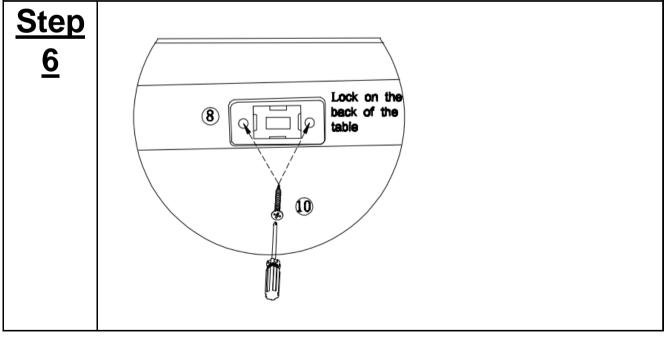
Use a Screwdriver (6) to lock the Bracket (8) with screws(10) to the back of the desk.
