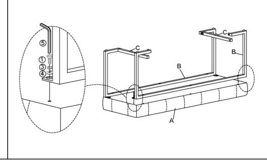
Place the other Metal Leg(B) on the Bottom of Bench Base(A) and attach where indicated above using Bolts(①), Spring Washers(③) and Washers(④) with the Allen Wrench(⑤).
