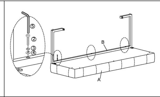
Further Attach Metal Leg(B) to Bench Base(A) where indicated using Bolts(②), Spring Washers(③) and Washers(④) with the Allen Wrench(⑤).
