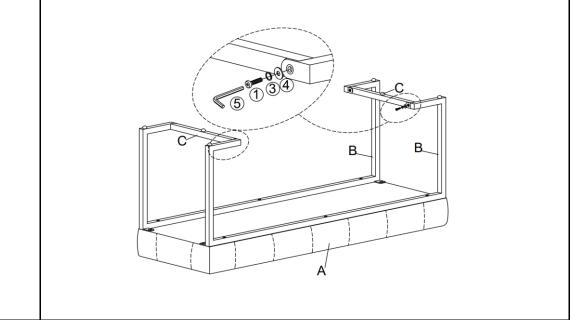
Using Bolts(①), Spring Washers(③), and Washers(④) with the Allen Wrench(⑤) connect the Metal Leg(B) to Iron Pipes(C).
