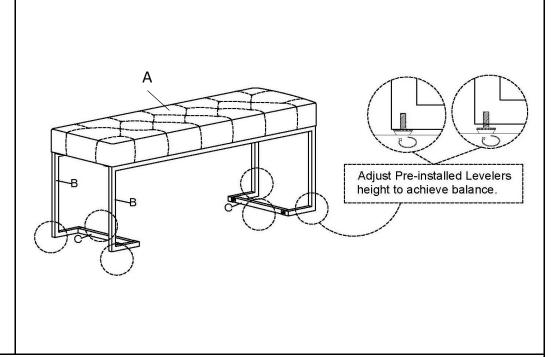
With assistance from an adult partner, stand the Bench up. Adjust the Pre-installed Levellers at the bottom of the Metal Legs(B) until the Bench is level with the ground.
