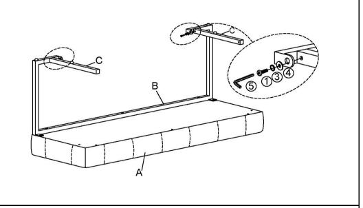
Using Bolts(①), Spring Washers(③), and Washers(④) with the Allen Wrench(⑤) affix the Iron Pipes(C) to the Metal Leg(B).
