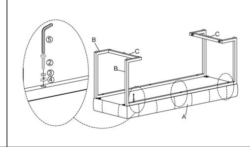
Further Attach Metal Leg(B) to Bench Base(A) where indicated above using Bolts(②), Spring Washers(③) and Washers(④) with the Allen Wrench(⑤).
