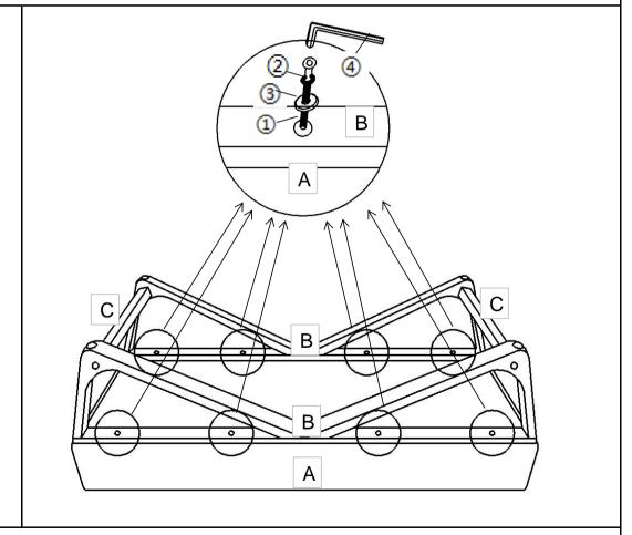
Attach Bench Seat(A) to Frame using Bolts(①), Spring Washers(②) and Washers(③) with Allen Key(④).
