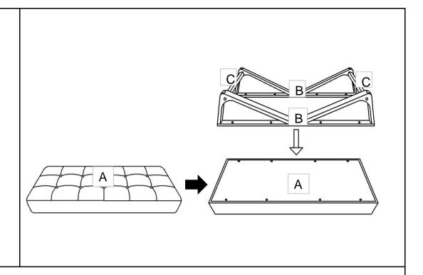
Place the Bench Seat(A) facedown onto a clean, non-marring surface. Align the mounting positions on the Side Frame(B) to those on the underside of Bench Seat(A), as pictured.
