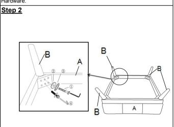
Insert one Wooden Leg(B) into the mounting position of the Ottoman(A).
