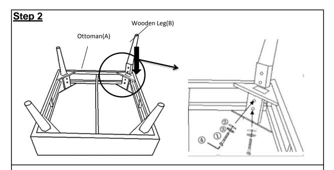
Insert one Wooden Leg(B) into the mounting position of the Ottoman(A). Attach using Bolts(1), Spring Washers(3) and Washers(2) with Allen Key(4). **Do not fully tighten the Bolts.**
