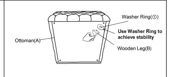
Install the first leg(B) into the bottom of the Ottoman(A) by placing 1 (ONE) piece of Washer Ring on the threaded stem.
