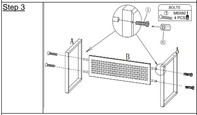
With assistance from your adult partners, Attach the two Metal Legs(A) to Metal Connection Board(B) using Bolts(1) with Screwdriver (6) At this stage, Do not fully tigthen Bolts .
