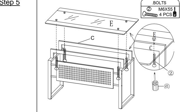
Attach Glass Table Top(E) to Metal Support Tubes(C) using Bolts(2) with Screwdriver(6)
