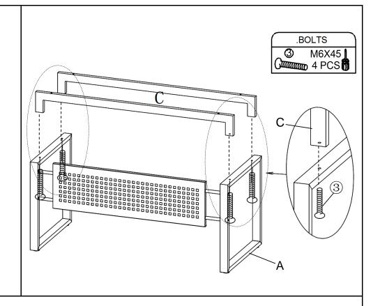
Attach two Metal Support Tubes(C) to two Metal Leg(A) using Bolts(③) with Screwdriver(6)
