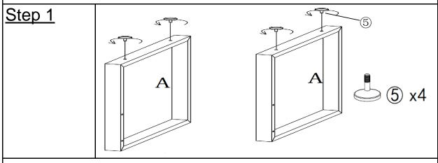
Screw-in the four Adjustable Glider Feet(⑤) into the bottom of the two Metal Legs(A) by hand.
