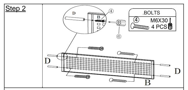
Attach four Metal Tubes(D) into Metal Connection Board(B) using Bolts(4) with Screwdriver(6)
