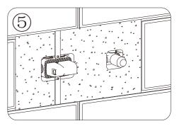
Make sure again that the pipe connection is correct and there is no leakage in the water test. Seal and fix the embedded box and pipe with packing. At this point, the solid wall embedded box is installed and the plastic protective cover is taken out.
