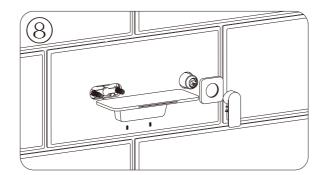
Install the water control switch and install the waterfall outlet as shown.
