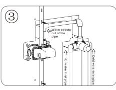
As shown in the figure, pre-bury the intake water pipe and pay attention to the preparation the upper and lower left and right directions of the buried box, the outlet is upward,connect hot water pipe on the left and cold water pipe on the right.
