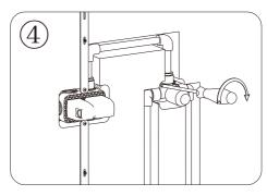
Open the water source to test whether the left and right inlet pipes are tightly connected without leakage. After the inlet pipes are tested and closed, adjust the flow switch to be in the open state to test whether the mixed outlet pipes are tightly connected without leakage. Adjust the horizontal position and fix it with the fixing bracket.
