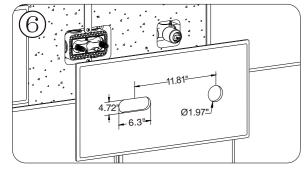
As shown in the picture, prepare to paste ceramic tiles. Open holes with a diameter of 1.97" on the right side and a gap of 4.92" between the two holes.Rectangular slot on the left side, center distance 11.81".
