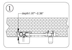
According to the basic size of the embedded box, use a special tool to cut the main hole on the solid wall between 1.97" and 2.36" deep.
