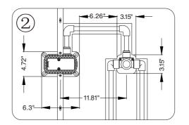
First find a good stainless steel fixing bracket, with crews locked in the embedded box up and down the xtended position; Wall pre (main body size 3.15"X3.15", outlet nozzle 6.3"X4.72").
