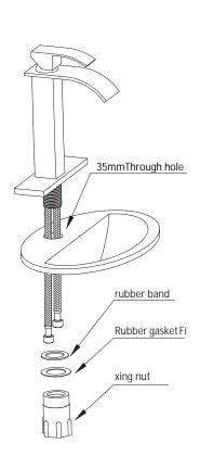
2 Make sure the basin has a  $\,$  35mm through hole, pass the hose through the hole, pass the rubber ring, rubber washer, and fixing nut into the hose in the order of the drawing, and tighten the fixing nut and the fixing screw to fix the faucet on the basin
