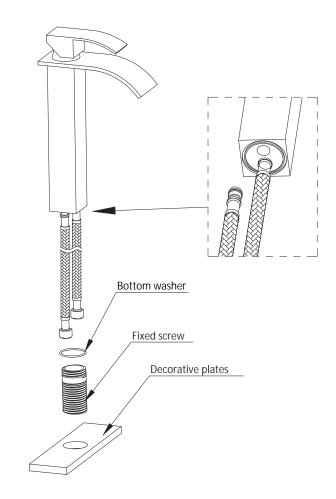
1、Connect the water inlet pipe to the faucet, then put the bottom gasket into the bottom of the faucet, then tighten the faucet with a fixing screw, and then put on the decorative panel.
