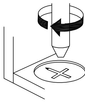
**EN**\_Turn cam lock clockwise to tighten.
