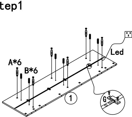
The led lamp is pasted in the groove and fixed with the snap.
