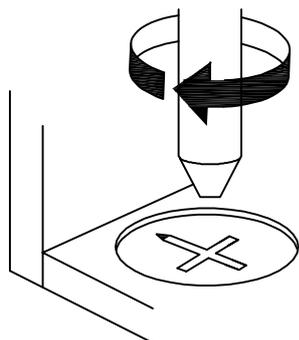
**EN\_Turn** cam lock clockwise to tighten.
