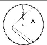
1.Screw a cam bolt A into the panel
