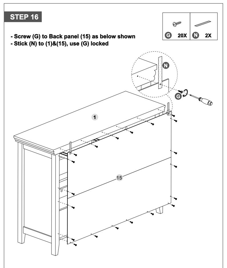
Warm Tips: ① It is recommended to put the product upside down When installing the back panel.
