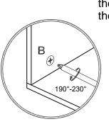
2.Push a cam B into the panel, make sure the arrow feature on the cam B points to the panel edge
