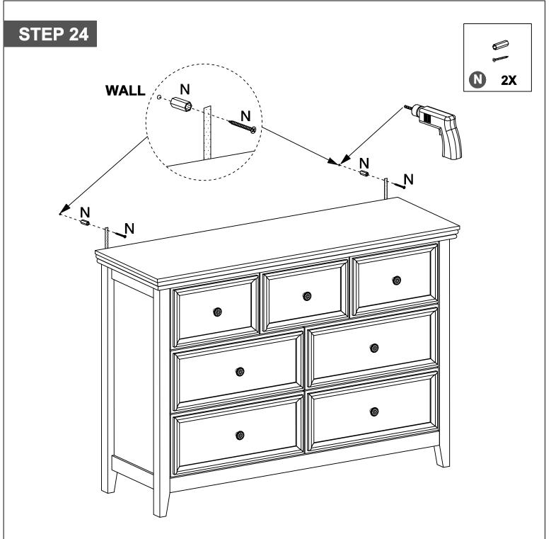
Tools required (not included): screwdriver, stud finder, tape measure, pencil, power drill and 3/16" drill bit.
