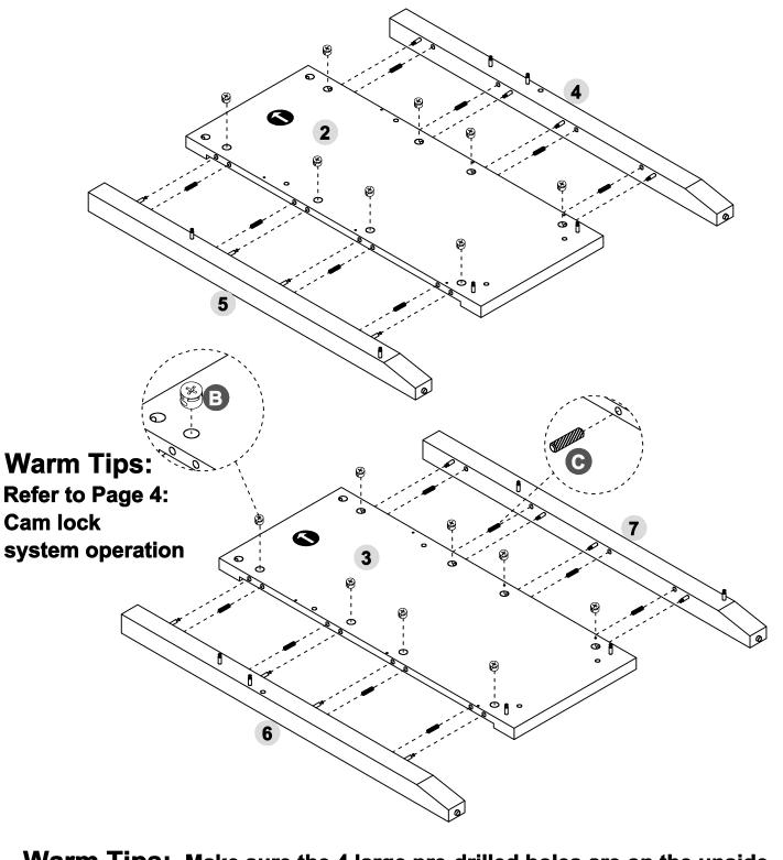
Warm Tips: Make sure the 4 large pre-drilled holes are on the upside, (4)&(5) holes should be in the same side.
