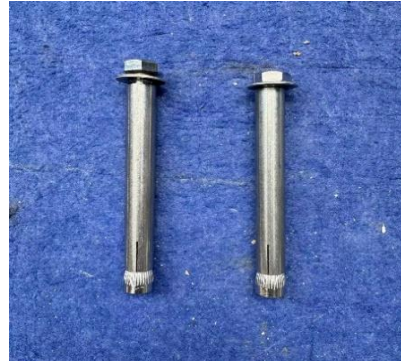
Photo.2 The masonry screws which were used to install the specimen to conduct the Resistance to Snow Load Test.
