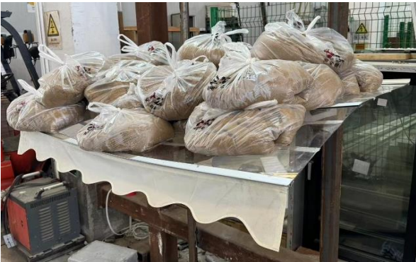
Photo.1 The Resistance to Snow Load Test on the testing specimen
