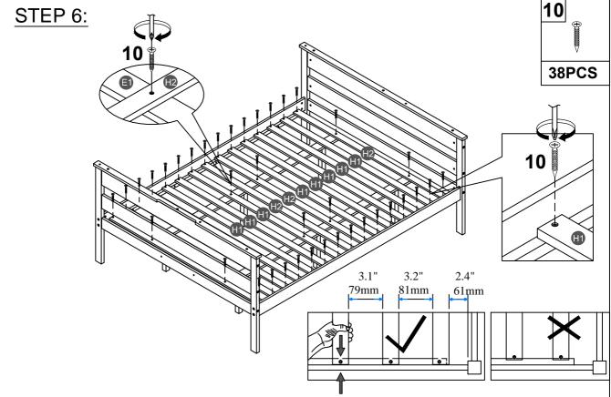
**NOTE:** Please make sure the bed slats close to the side rail before locking the screws to avoid breakage. This step is required for both the left and right sides. Moreover, please do not lock the screws of the bed slats at the outermost edge to avoid damaging.
