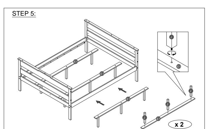
Assembling leg support (J) with lower support slat (E1) later rotate, Move support slat inside bunkbed.
