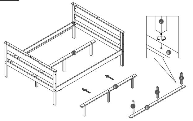
Assembling leg support (J) with lower support slat (E1) later rotate, Move support slat inside bunkbed.
