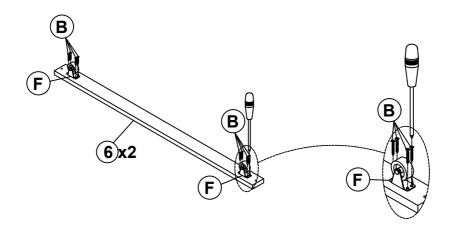
Step 5 First attach 2pcs part 6 to the front and end of the frame, between side rails. Then attach the remaining part 6 equidistantly between side rails.
