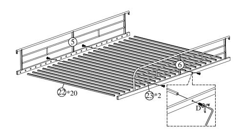
NOTE: In this step, DO NOT tighten any bolt until you connect all part together
