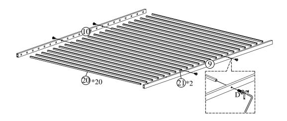
NOTE: In this step, DO NOT tighten any bolt until you connect all part together
