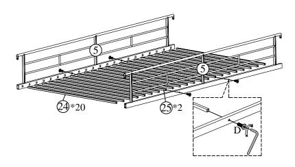
NOTE: In this step, DO NOT tighten any bolt until you connect all part together
