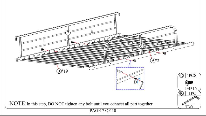
$STEP\ 4$  : Following below illustration Assembly Frame #4. Using hardware #D connect #8 with #9, #10 to complete Frame #4.
