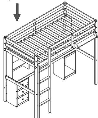
Make sure to tighten all the screws of the bed.
