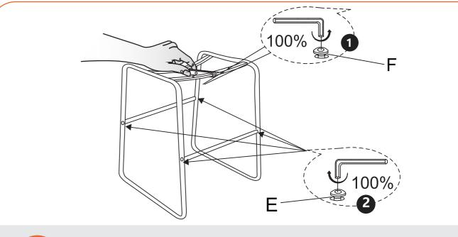
Adjust the connection between legs (B) and (C) to make it flat. Then, 100% tighten the Bolts in the order shown.  $F \rightarrow E$
