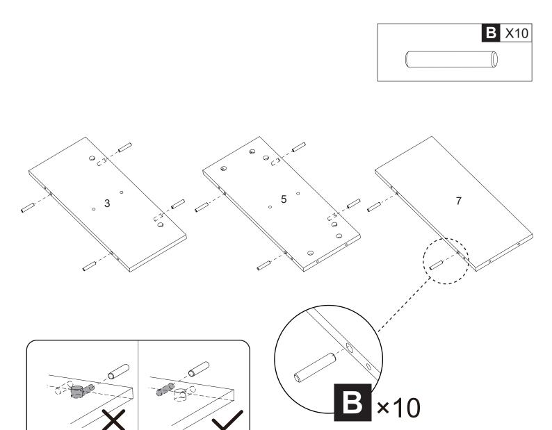
Attach Wooden Pin (B)\*10 to Board (3), (5) and (7).
