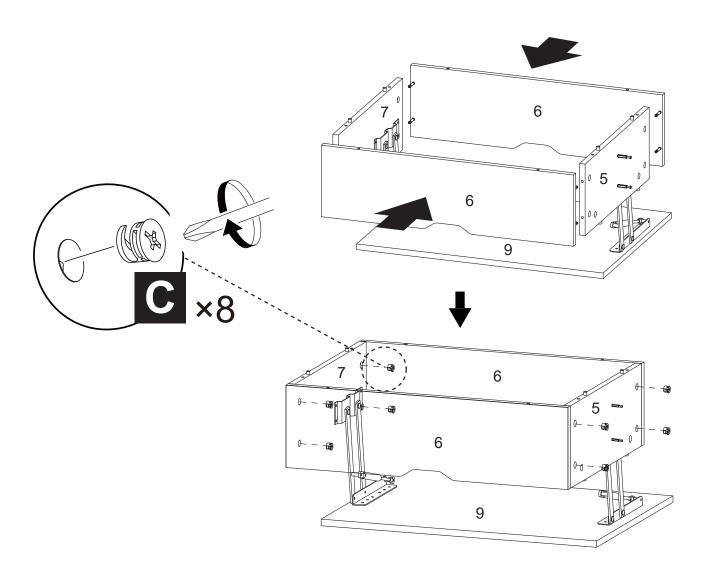
With the notched side of Board (6) facing down, install Board (6)\*2 to Boards (5&7) with Eccentric Wheel (C)\*8.
