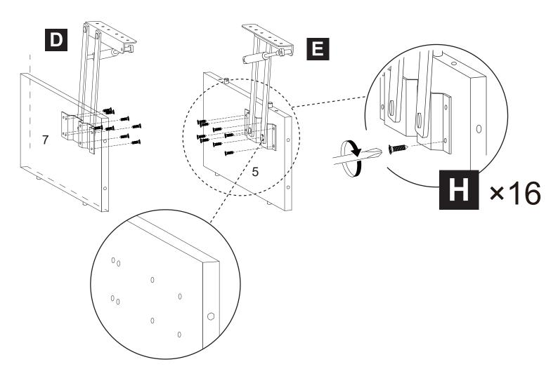
Using Bolts (H)\*16, install Left Lifter (D) to the pre-drilled holes on the inside of Board (7), and Right Lifter (E) to the pre-drilled holes on the inside of Board (5).
