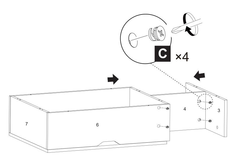
As shown, install Board (4) to Board (5), and install Board (3) to Board (4) with Eccentric Wheel (C)\*4.
