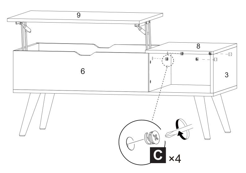
Tighten Eccentric Wheel (C)\*4 and make sure Board (8) is fixed.
