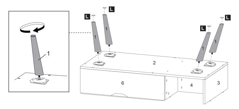
Tighten Wooden Leg (1)\*4 completely, and glue Silicone Foot Pad (L)\*4 on the bottom of it.
