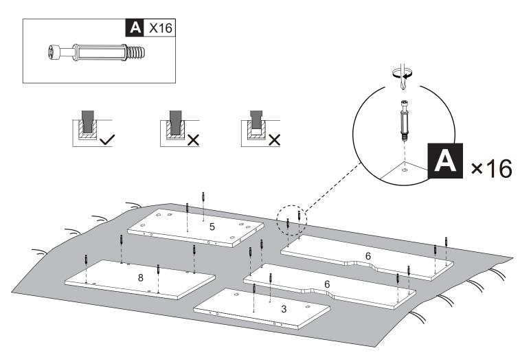
Fix Derrick Screw (A)\*16 to Board (3), (5), (6)\*2, (8) as shown.
