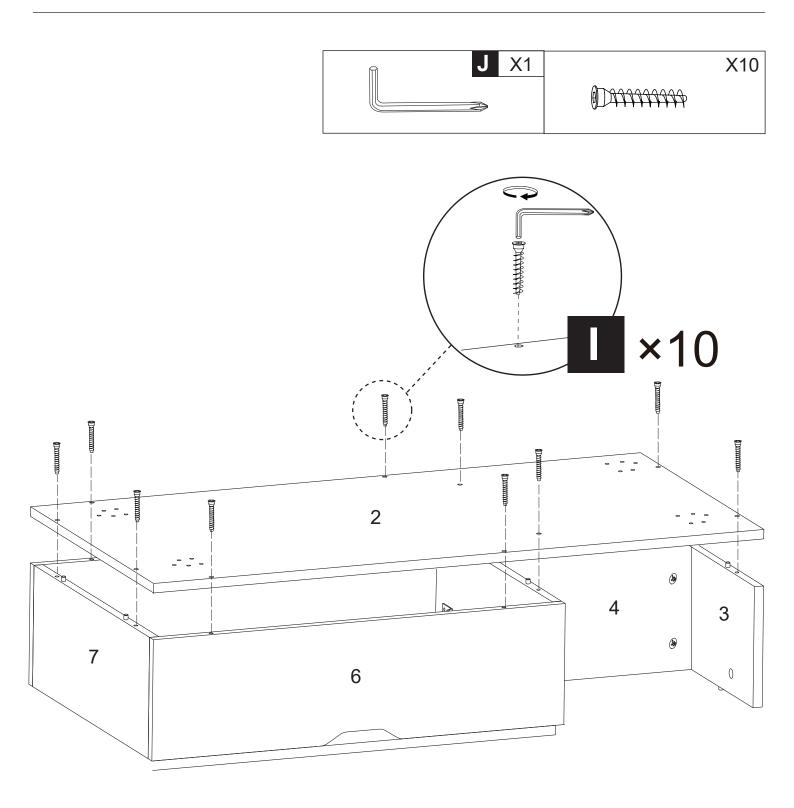
Using Wrench (J), install Board (2) to the completed frame with Bolts (I)\*10.
