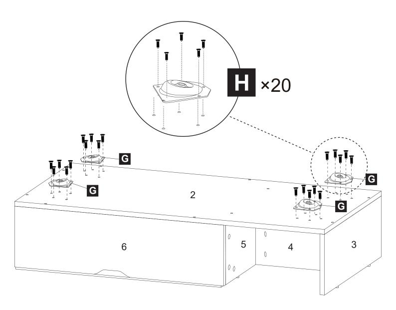
Using Bolts (H)\*20, install Solid Wood Foot Connector (G)\*4 to the four corners of Board (2).
