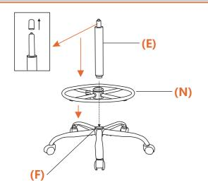
Insert Gas Lift (E) into the center hole of the Foot Ring (N) and lift the Foot Ring upward to secure it to the Gas Lift. Then insert Gas Lift (E) into the Base (F). Remove the cover from the top of the Gas Lift (E).
