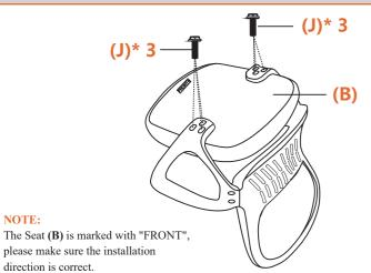
Turn the Seat (B) upside down . Using Wrench (M), install Armrests (C)\*1L\*1R to the Seat with Bolts (J)\*6.
