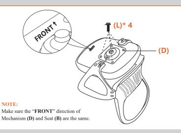
Using Wrench (M), attach Mechanism (D) to the Seat (B) with Bolts (L)\*4.
